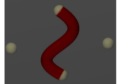
Deformed vessel by moving the control points
